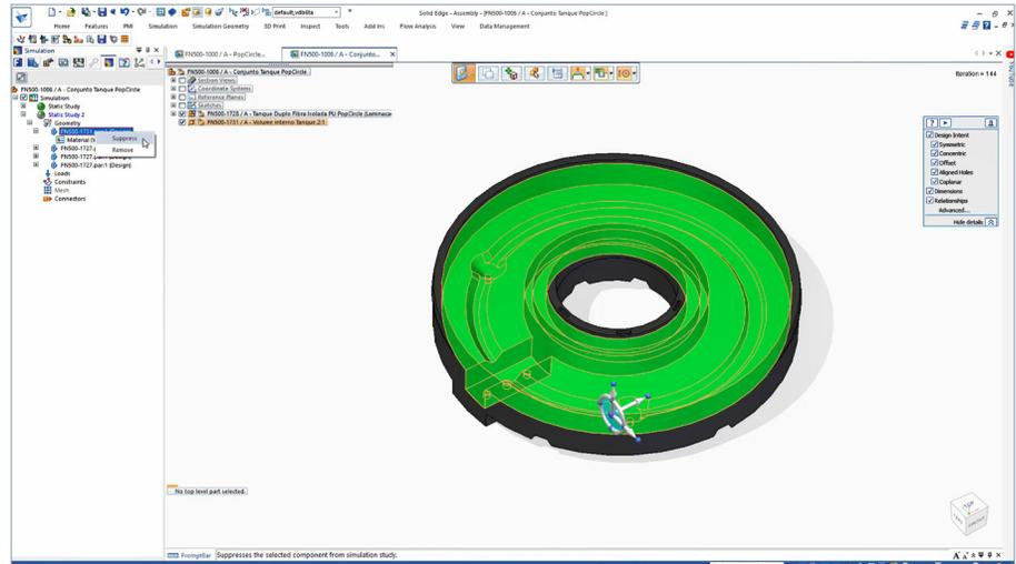
rotation, symmetric and cylindrical variations. The loads are also geometry-based and include mechanical as well as temperature loading for thermal analyses. Mechanical loads include forces, pressures and effects caused by body rotation and gravity. Solid Edge Simulation facilitates load and constraint applications with Quick Bar input options and handles for direction and orientation definition.
